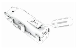
2. Insert the SCM into the compartment top first, then snap the bottom into place.
